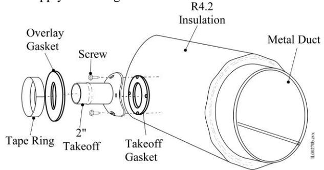
Figure 3 Metal Plenum Takeoff Installation
