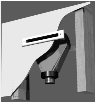
Figure 2. Typical Wall Installation, 90° Outlet
