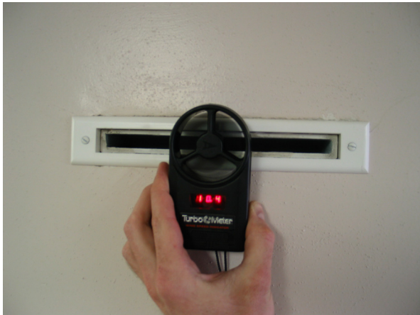
Figure 7. TurboMeter Placement for Slotted Outlets
