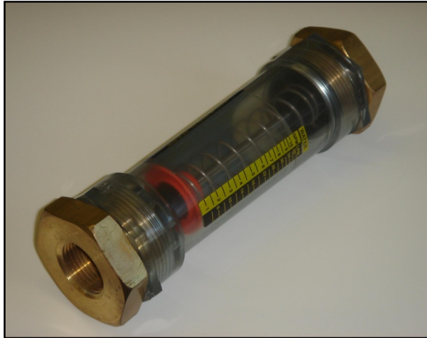
Figure 1. Shuttle-Type Inline Flowmeter.
