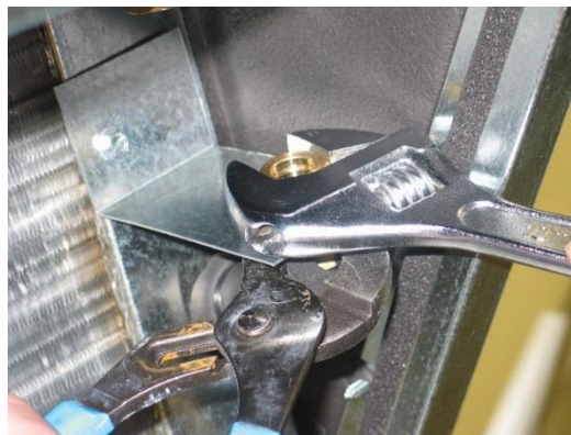
Figure 22. (Step 1) remove nut as shown.
