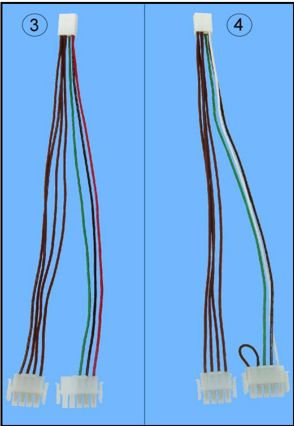
Figure 9. Motor Harness: (3) 208-230V, (4) 110V
