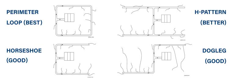
• **60/40 Rule.** When using a tee split the flow as close to 50/50 as possible — no more than 60/40. Always use a turning vane.
