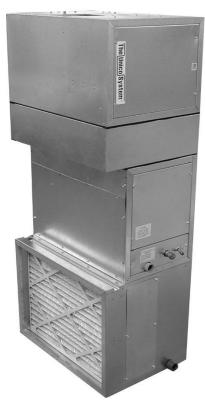
light enough for one person to install. They can be arranged in a horizontal, upflow, or downflow configuration. There are three basic modules: a cooling module (refrigerant or chilled water coil), a heating module (with hot water coil), and a blower module (with controls). The unit may be matched with most conventional condensing units or heat pumps of proper capacity.
