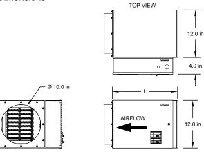
SIDE VIEW 10.0 in. Round plenum adapter shown attached (Supplied). Optional: 9.5 in. x 9.5 in. square plenum adapter (Supplied) is shipped loose. IL00002(Rev D).cvx
