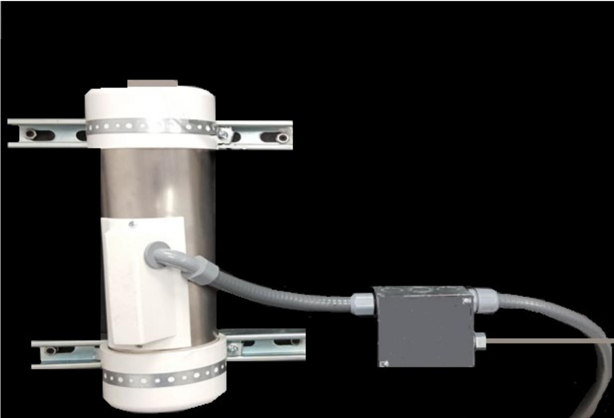
Shown above: V18 mounted on a painted plywood board with Uni-struts. Or mount to other wood mounting, not metal. Flow must enter from the bottom, plastic cover should be closer to the bottom as shown
