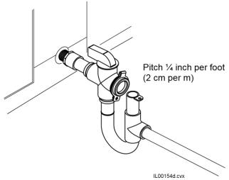
Figure 20. Typical Condensate Trap
