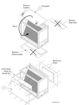
Figure 7. Cooling Module Configuration (2430, 3036, 3642 only)
