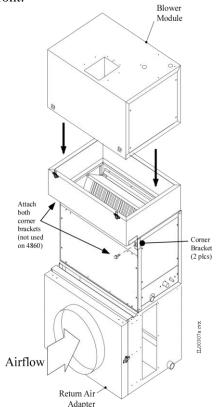
Figure 10. Installing the Blower Module
