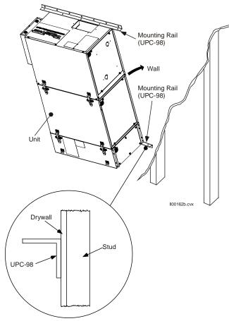
Figure 14b. Typical Vertical Mounting
