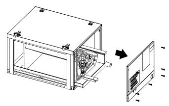
Figure 37. Removal of M1218 Cooling Coil
