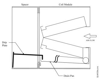
Figure 5. 4860 Drip-plate installation (horizontal)
