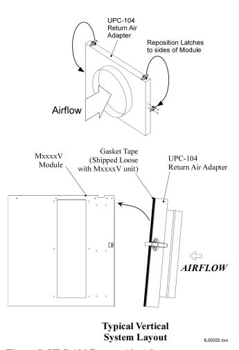
Figure 8. UPC-104 Return Air Adapter Installation
