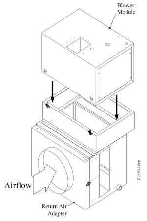
Figure 11. Heating-Only Vertical Modular System
