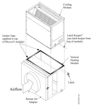
\*Note: Attach Latch keeper to opposite side (not shown)
