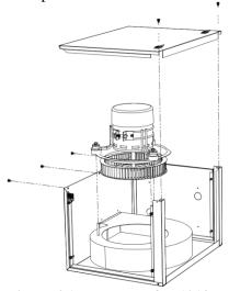
Figure 36. Removal of M1218 Motorized Blower Assembly
