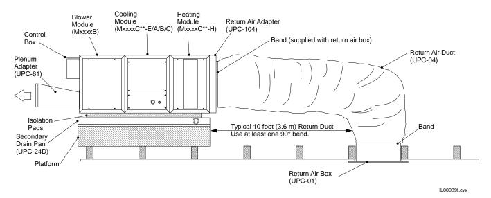
Figure 3. Typical Horizontal Attic Installation
