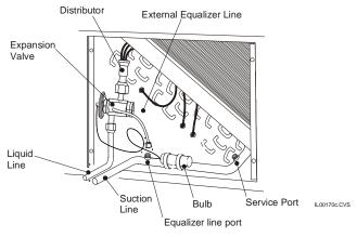
Figure 21. 1218 Expansion Valve Location
