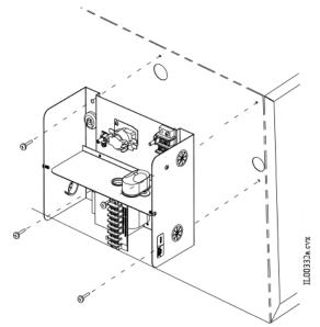
Figure 12. Control Box Mounting
