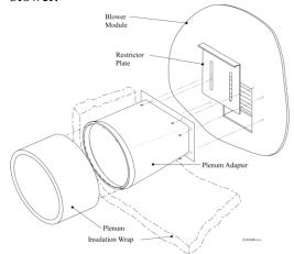
Figure 17. Supply Plenum Adapter Installation
