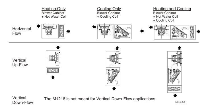
Figure 2b. Basic Module Arrangement for 1218
