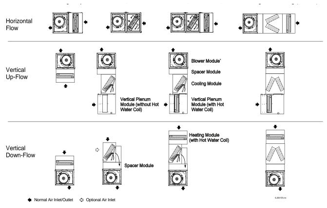
Figure 2a. Basic Module Arrangement (2430, 3036, 3642, and 4860)
