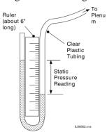
Figure 34. U-Tube Manometer
