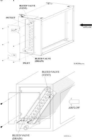
Figure 32. Water Coil Connections Coil Cleaning.
