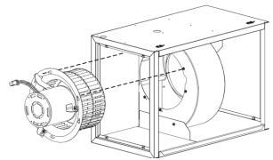
Figure 35. Removal of the Motorized Blower Assembly
