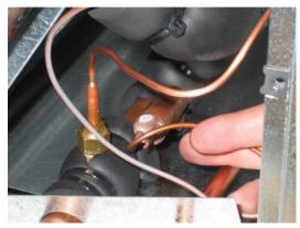
Figure 29. Thermal Measuring Bulb Placed on Copper Tube.
