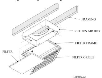
Figure 19. Return Air Box and Filter
