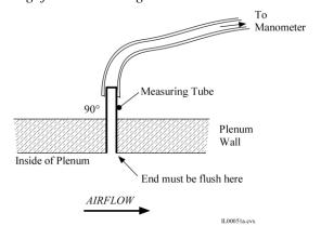
Figure 33. Measuring Plenum Static Pressure
