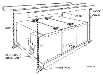
Figure 14a. Typical Suspended Mounting
