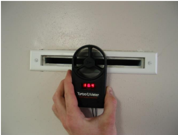
Figure 8. TurboMeter Placement for Slotted Outlets
