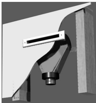
Figure 3. Typical Wall Installation, 90° Outlet
