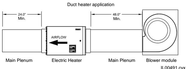
Allow at least 25-inches (610-mm) in front of the control for servicing. External insulation is required for high humidity applications (refer to the installation bulletin for more information).
