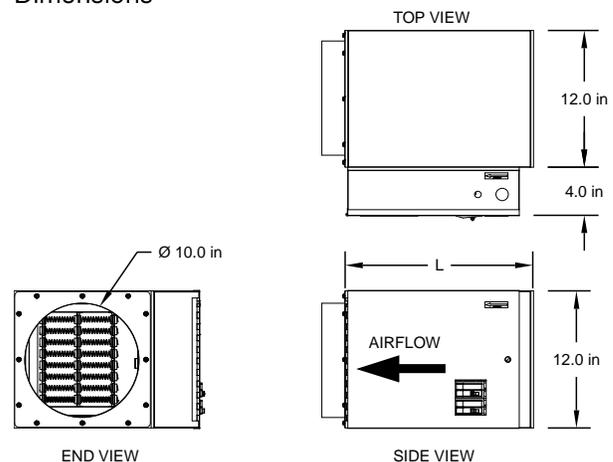
10.0 in. Round plenum adapter shown attached (Supplied). Optional: 9.5 in. x 9.5 in. square plenum adapter (Supplied) is shipped loose.
