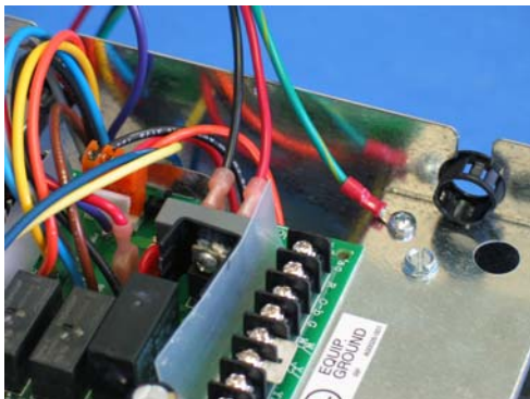
Connect ground wire to control box with sheet metal screw.
