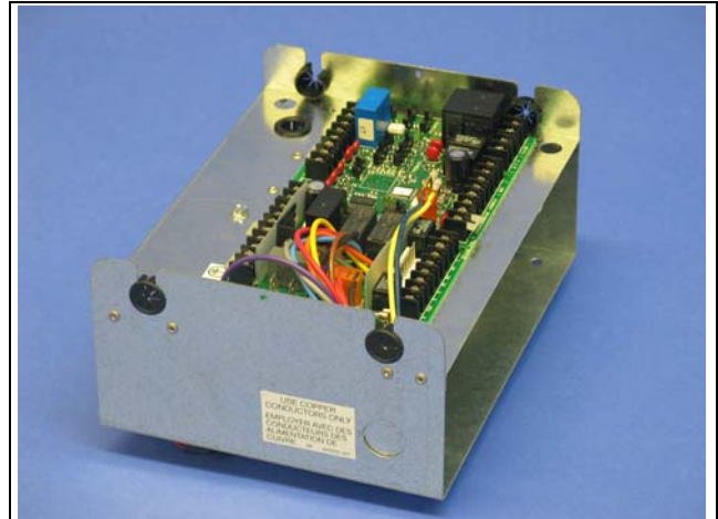
Figure 1. Advanced control board in control box
