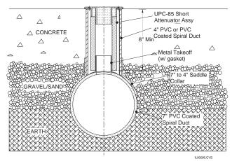
Figure 2. Typical Slab Installation
