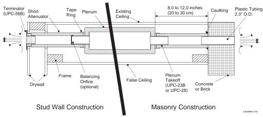
Figure 1. Typical Corridor Installation
