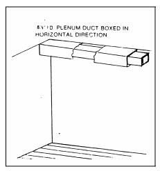
Figure 7. Typical Plenum Horizontal Layout
