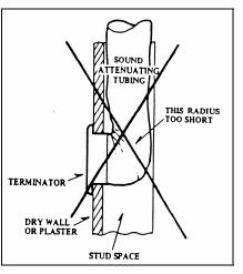
Figure 11. Incorrect Placement of Tubing
