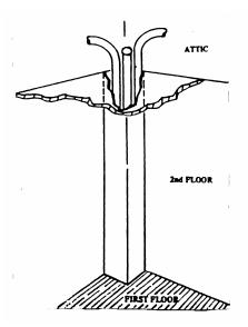
Figure 13. Placement of Supply Tubing between Floors
