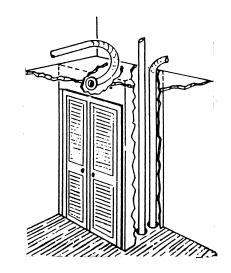
Figure 15. Placement of Supply tubing
